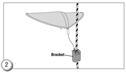
• Fit an end of the canopy stay into the socket in a bracket. **Hint:** The long end of the canopy should face the front of the swing.
